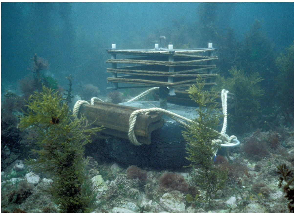
Figure A.1: Example of a crevice collector used to monitor the settlement rate of puerulus stage red rock lobster around New Zealand. Image reproduced with permission from John Booth.
